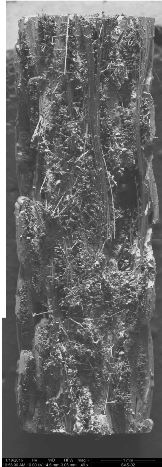
Figure 37. SEM micrograph of fracture surface of the specimen tested in tension to failure at 1300 °C.
