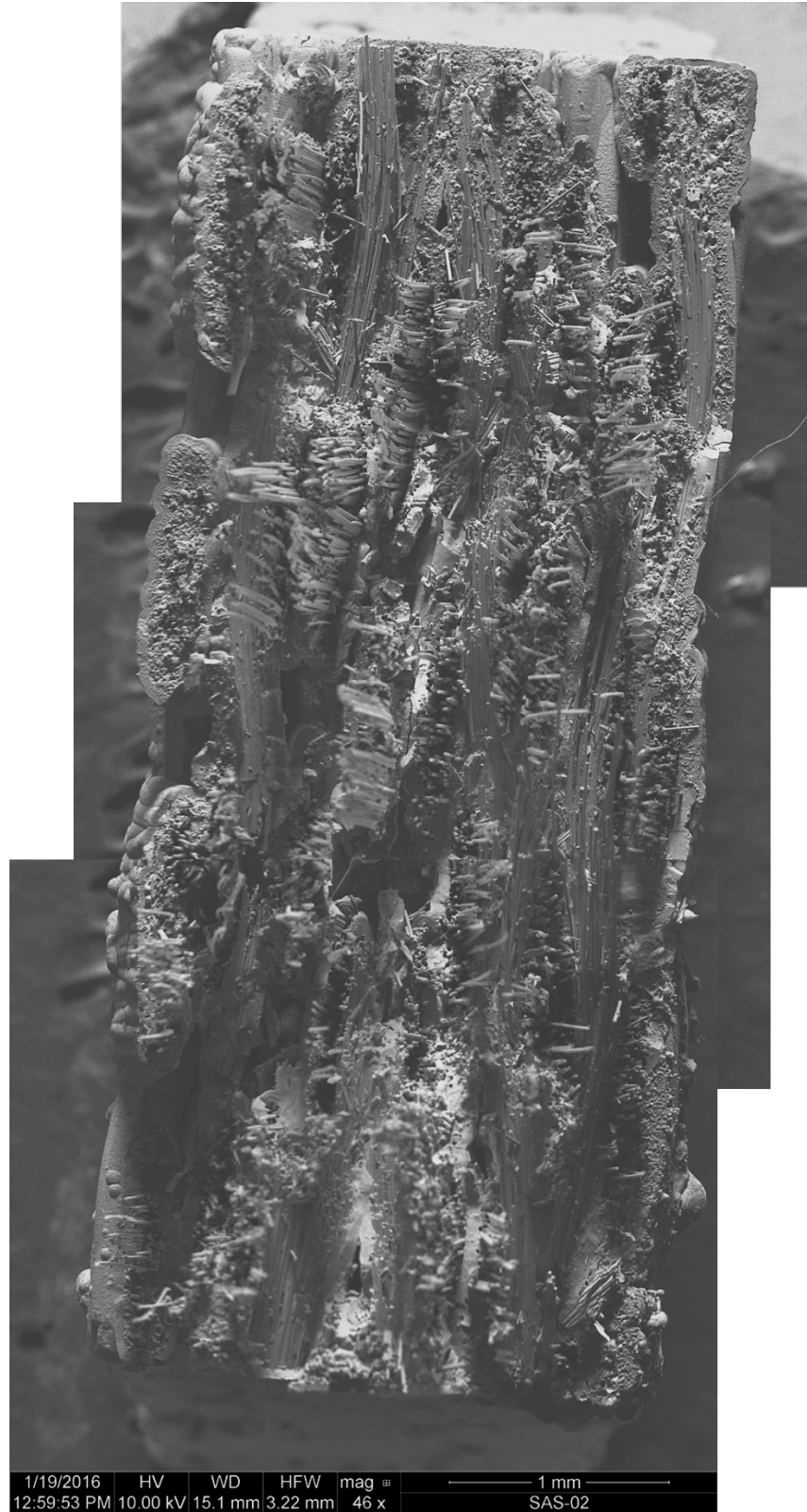
Figure 106: Fracture surface of the HG-shaped specimen tested in fatigue at 1300°C in steam, \sigma_{\max} = 100 MPa, N_f = 200,000 , t_f = 55.6 h.
