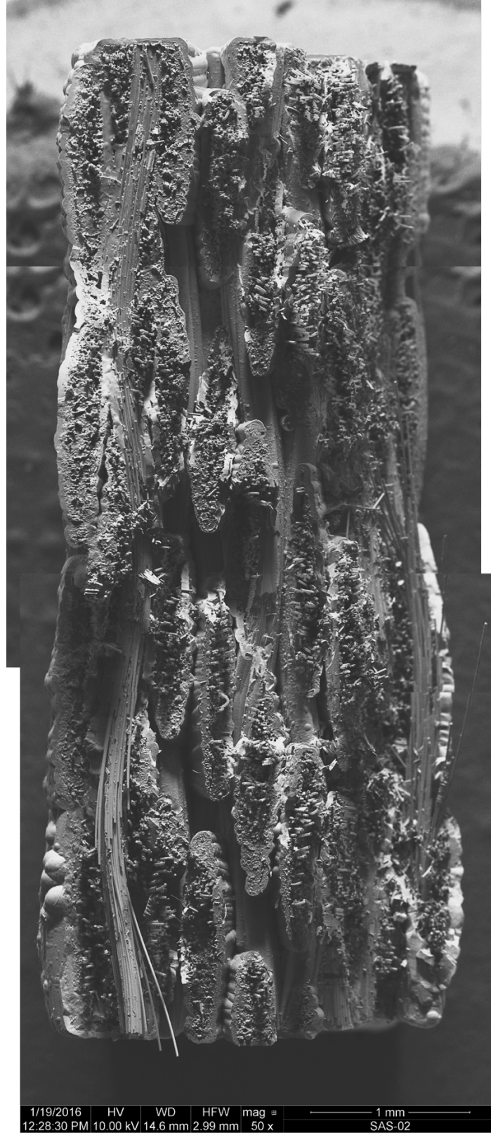
Figure 104: Fracture surface of the HG-shaped specimen tested in fatigue at 1300°C in steam, \sigma_{\max} = 150 MPa, N_f = 13,266 , t_f = 3.7 h.
