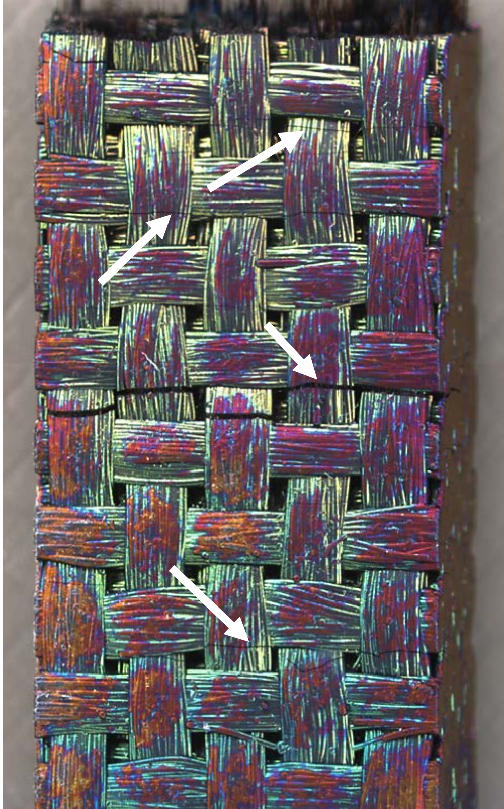
Figure 47. Gage section of the DB-shaped specimen tested in fatigue at 1300°C in air, \sigma_{\max} = 140 MPa, N_f = 20,069 , t_f = 5.6 h. Transverse cracks of the 0° fiber bundles are visible on the specimen surface.
