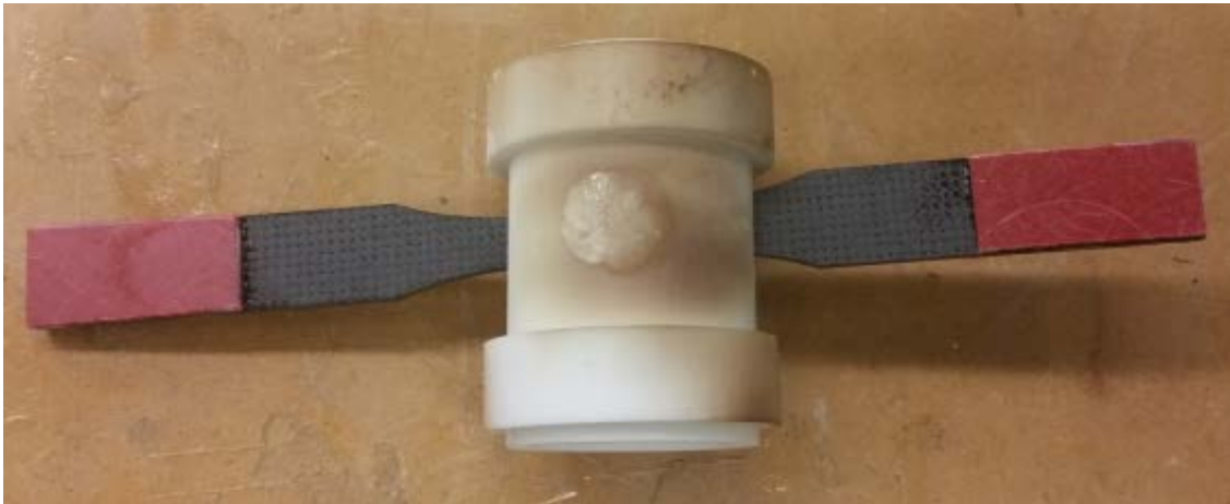
Figure 14. Test Specimen with alumina susceptor.
