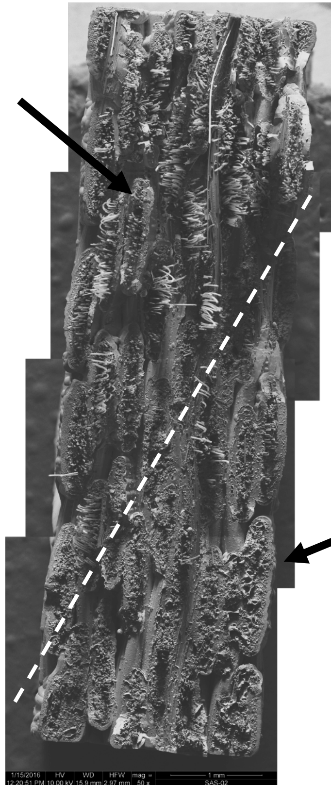
Figure 94: Fracture surface of the DB-shaped specimen tested in fatigue at 1300°C in steam, \sigma_{\max} = 140 MPa, N_f = 72,074 , t_f = 20.0 h.
