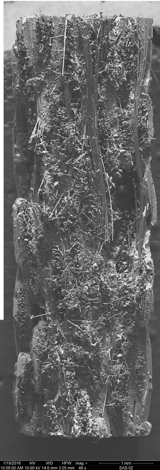
Figure 80: Fracture surface of the specimen tested in tension to failure at 1300 °C.
