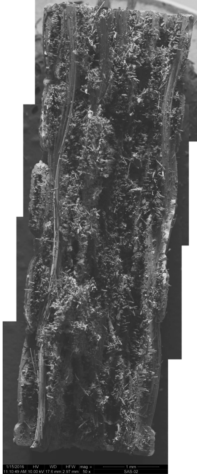
Figure 90: Fracture surface of the DB-shaped specimen tested in fatigue at 1300°C in air, \sigma_{\max} = 70 MPa, N_f = 200,000 , t_f = 55.6 h.
