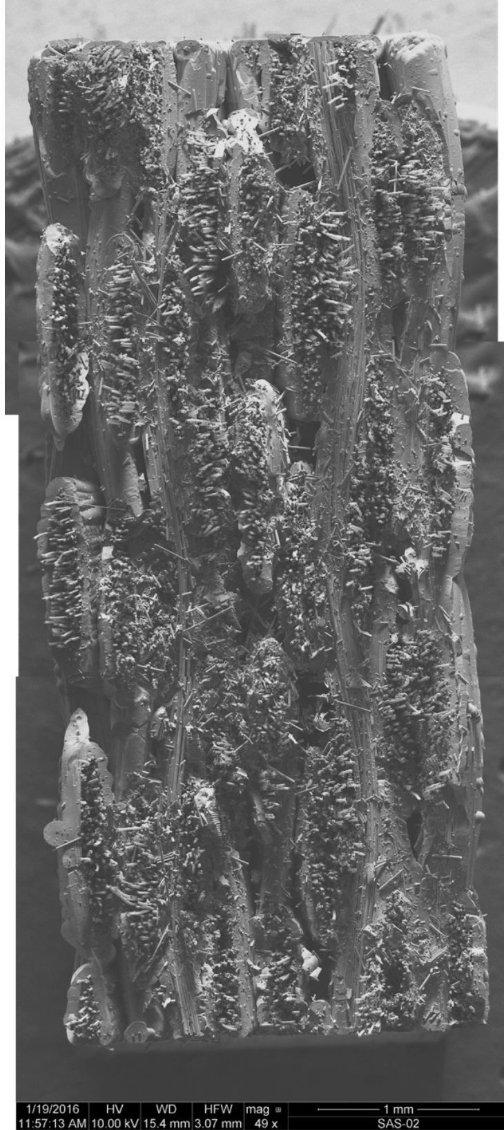
Figure 102: Fracture surface of the HG-shaped specimen tested in fatigue at 1300°C in air, \sigma_{\max} = 80 MPa, N_f = 200,000 , t_f = 55.6 h.
