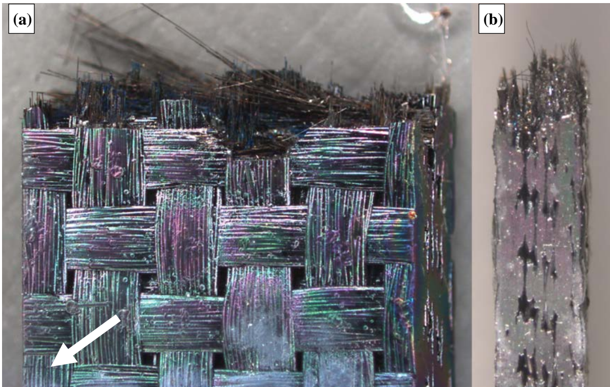
Figure 42. Optical micrograph of fracture surface of the DB-shaped specimen tested in fatigue at 1300°C in steam. \sigma_{\max} = 160 MPa, N_f = 17,811 , t_f = 4.9 h. (a) front, (b) side.
