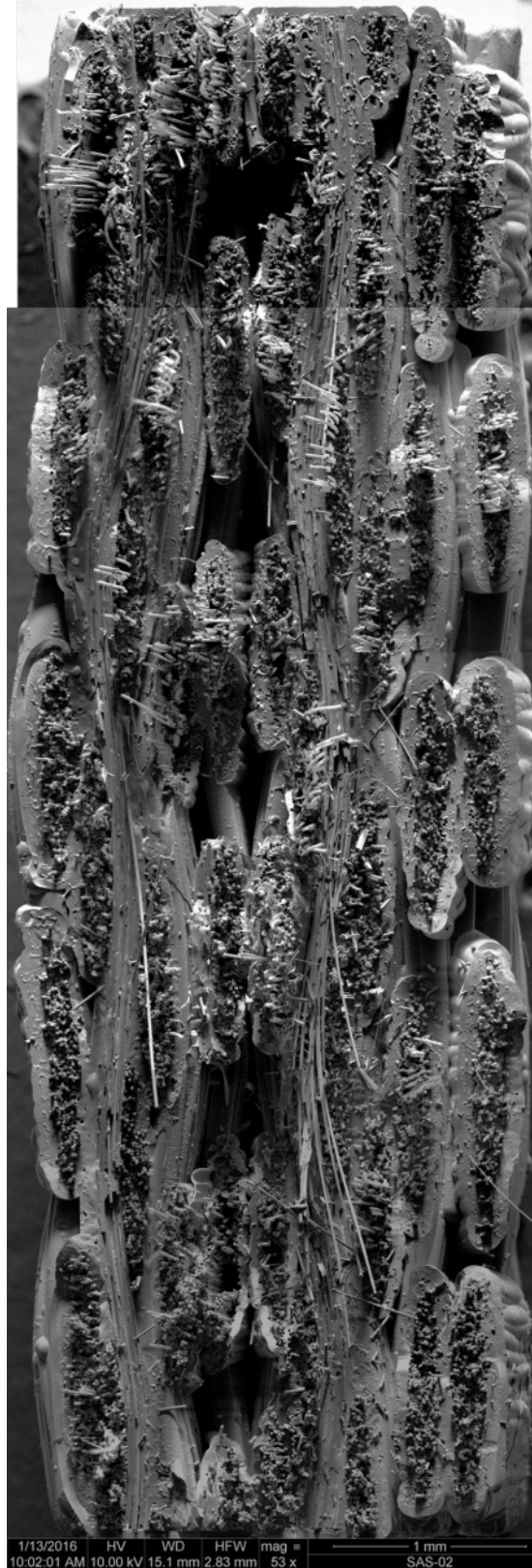
Figure 82: Fracture surface of the DB-shaped specimen tested in fatigue at 1300°C in air, \sigma_{\max} = 140 MPa, N_f = 20,069 , t_f = 5.6 h. Oxidation visible around the longitudinal fiber tows.
