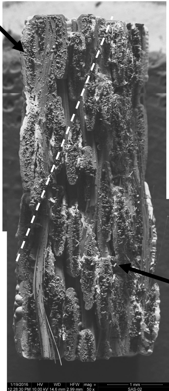
Figure 57. Fracture surface of the HG-shaped specimens tested in fatigue at 1.0 Hz at 1300°C in steam. \sigma_{\max} = 150 MPa, N_f = 13,266 , t_f = 3.7 h.
