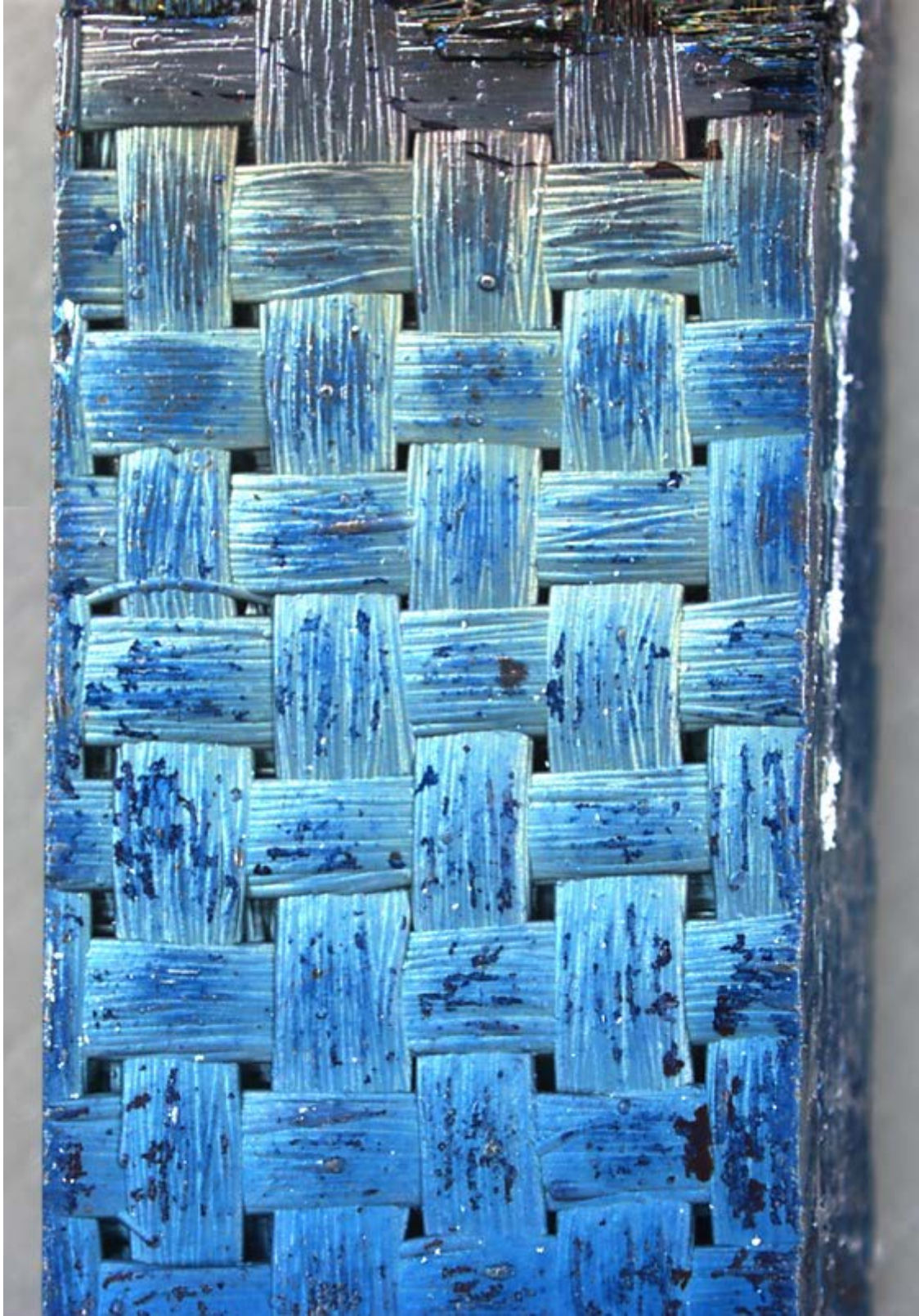
Figure 46. Gage section of the DB-shaped specimen L97, tested in tension to failure at 0.05 mm/s at 1300°C in air.
